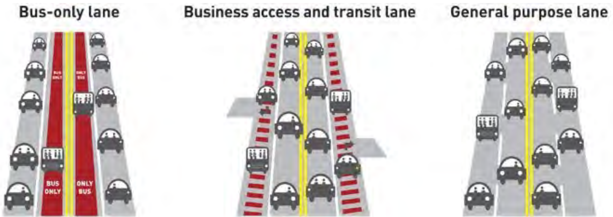
Figure B.1 BRT Guideway Treatments
