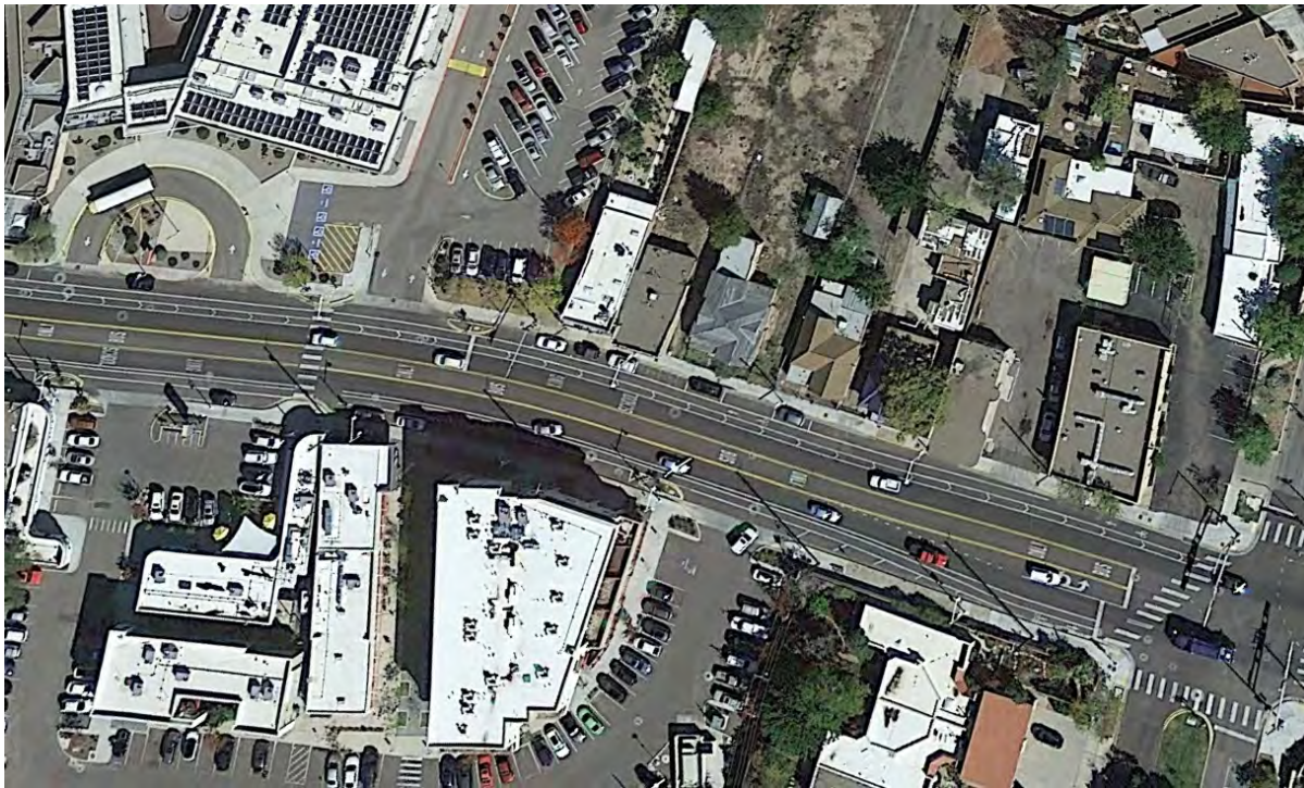
Figure B.10 Reversible Lane Section (between Yellow Lines) in Albuquerque, New Mexico Source: Google Earth
