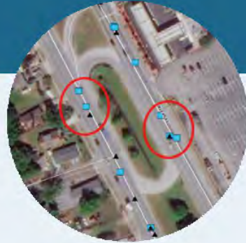
Median U-Turn Acceleration/Merge Lanes
